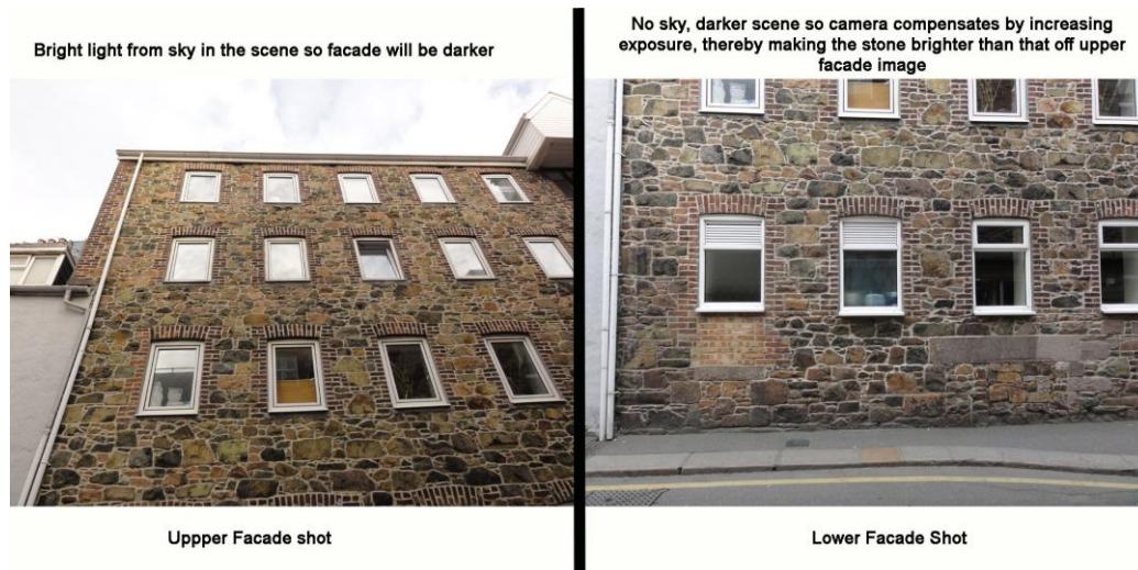
Figure 5: Variable exposure on façade when using auto exposure.
